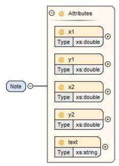
This element defines a graphical note to be placed on the canvas of the enclosing system. It is sized using the attributes so that the coordinates (x1,y1) and (x2,y2) define the positions of the lower-left and upper-right corners of the note in the coordinate system of the parent.
