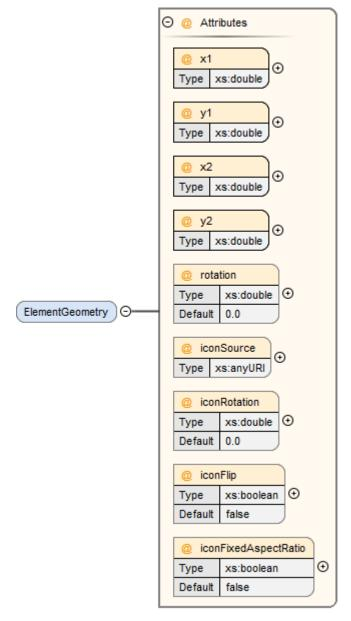
This optional XML element defines the geometry information of the model element, where (x1,y1) and (x2,y2) define the positions of the lower-left and upper-right corners of the model element in the coordinate system of its parent system. If x1>x2 this indicates horizontal flipping, y1>y2 indicates vertical flipping.
