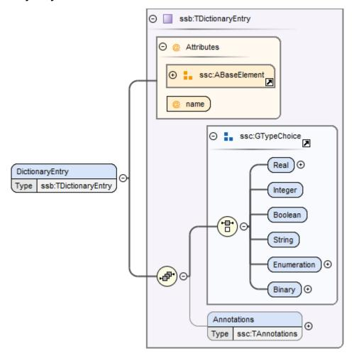
A dictionary entry defines a single signal in the signal dictionary.
