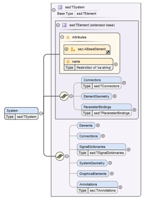
This element describes a system, which can contain components, signal dictionary references and other systems as elements, connectors as an interface to the outside world, and connections connecting the connectors of itself and of its elements to one another.
