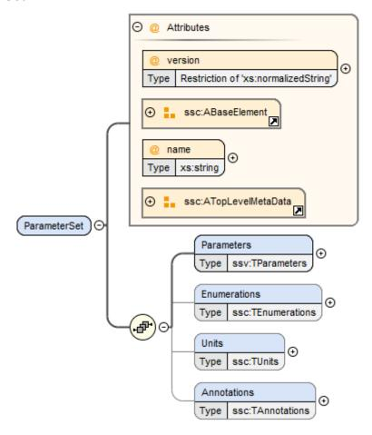
The ParameterSet element contains parameter and meta data information. If the SSV is provided as a separate file, the root element MUST be a ParameterSet element.
