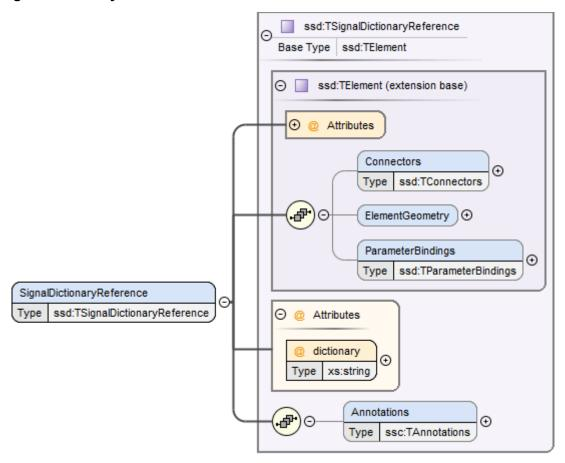
A signal dictionary reference is an element of a system that references a signal dictionary, i.e. it is the place-holder of the signal dictionary that allows access to the contents of the signal dictionary through its connectors, which **MUST** reference signal dictionary entries.
