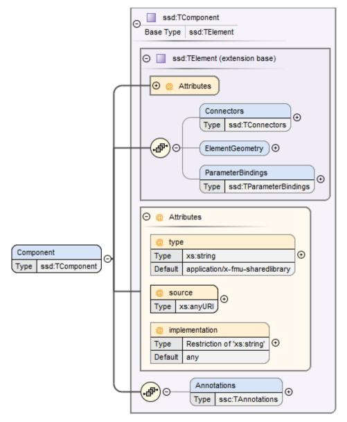
A component is an atomic element of a system (i.e. its internal structure is not specified).
