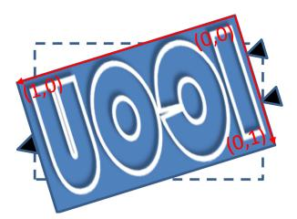
Example 15: Horizontal and vertical flip (x1>x2, y1>y2), rotation= $\varphi$  iconRotation= $\varphi$ , iconFixedAspectRatio=true, iconFlip=false
