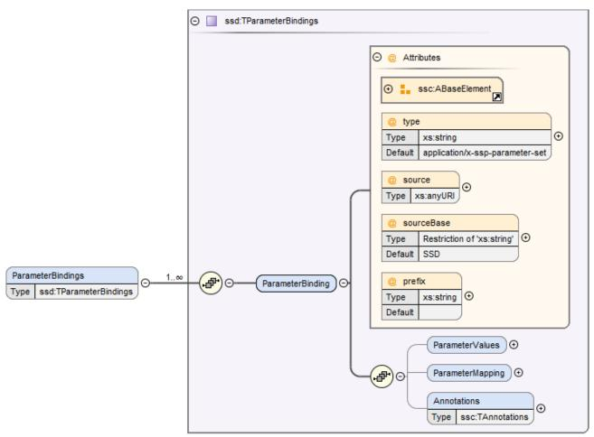
The ParameterBindings element provides the parameter bindings for a component or system, where each binding is specified in a ParameterBinding element. A parameter binding applies a set of parameter values (a parameter set), supplied by a parameter source (for example a parameter file) to parametrize a component or system.
