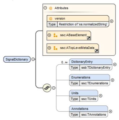
This element describes a signal dictionary, which consists of one or more dictionary entries, each describing one signal in the signal dictionary (see next section).
