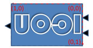
Example 13: Horizontal and vertical flip (x1>x2, y1>y2), rotation= $\varphi$  iconRotation= $\varphi$ , iconFixedAspectRatio=true, iconFlip=true
