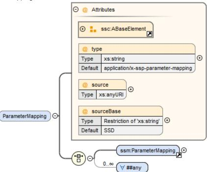
This element provides a parameter mapping, which specifies how the parameter names and values provided in the parameter source are to be mapped to the parameters of the component or system in question. If no mapping is supplied, the parameter names of the parameter source are used as is for name matching against the names of parameters in the component or system and the values of the parameter source are not transformed further before being applied.
