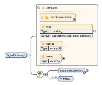
A signal dictionary is a collection of signals which can be accessed in different systems at different levels of the hierarchy through signal dictionary references referencing the signal dictionary.
