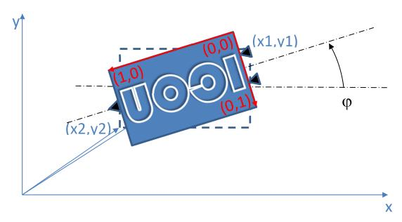
Example 14: Horizontal and vertical flip (x1>x2, y1>y2), rotation= $\varphi$  iconRotation= $\varphi$ , iconFixedAspectRatio=false, iconFlip=true
