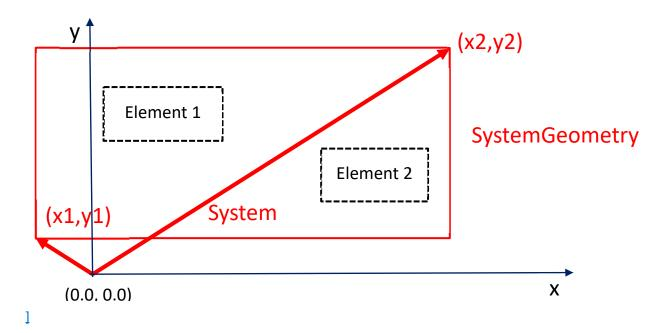
[ Graphical example showing the interplay of SystemGeometry, ElementGeometry, ConnectorGeometry, and ConnectionGeometry:
