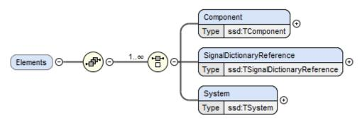
This optional element contains one or more components, signal dictionary references or systems that are the internal content of the given system.
