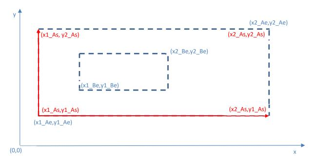
To plot the element B in the system where A is located, use the following coordinate transformation:
