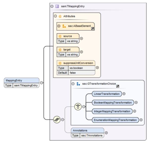
This element specifies a single mapping between a parameter in the source and a parameter of the system or component being parametrized. Through its optional GTransformationChoice element a transformation can be specified that is to be applied to the parameter value prior to its application to its target parameter.
