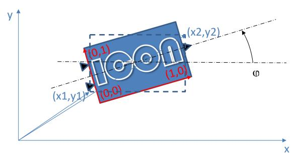
**Example 4: No flip (**x1<x2, y1<y2), rotation= $\varphi$
