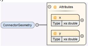
This optional XML element gives the geometry information of the connector. Note that x and y coordinates are in a special coordinate system, where 0,0 is the lower-left corner of the containing model element, and 1,1 is the upper-right corner of the model element, regardless of aspect ratio.
