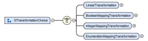
The following XML child elements specify a transformation to be applied to a value prior to its use in a connection or parameter mapping:
