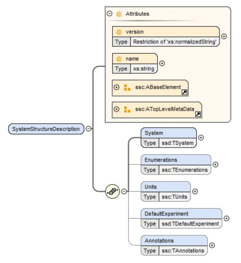
The root element of an SSD file **MUST** be a SystemStructureDescription element, which gives overall information about the system hierarchy described in this SSD file, including common meta-data, and acts as a bracket for the root system and its unit and enumeration definitions.
