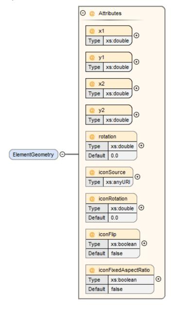
This optional XML element defines the geometry information of the model element, where (x1,y1) and (x2,y2) define the positions of the lower-left and upper-right corners of the model element in the coordinate system of its parent system. If x1>x2 this indicates horizontal flipping, y1>y2 indicates vertical flipping.
