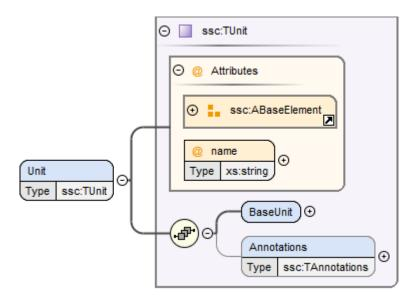
Each unit is defined through a Unit XML element:
