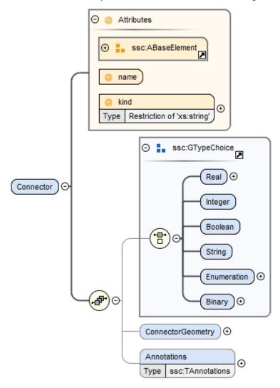
The following XML attributes are specified for the Connector element:
