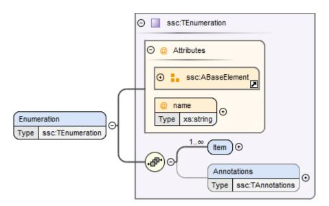
Each enumeration is defined through an Enumeration XML element:
