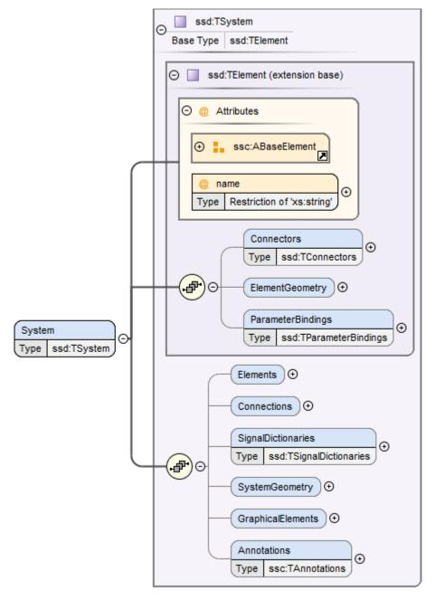
This element describes a system, which can contain components, signal dictionary references and other systems as elements, connectors as an interface to the outside world, and connections connecting the connectors of itself and of its elements to one another.
