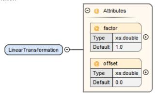
This element provides for a linear transformation of the source value to the target value, i.e. in the calculation target = factor \* source + offset.
