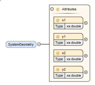
This element defines the extent of the system canvas. (x1,y1) and (x2,y2) define the lower-left and upper-right corner, respectively. Different from ElementGeometry, where x1 > x2 and y1 > y2 indicate flipping, x1 < x2 and y1 < y2 MUST hold here.
