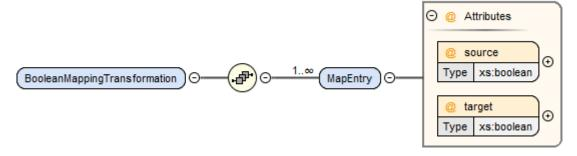
This element provides for a transformation of Boolean values based on a mapping table and is valid for connectors of Boolean type. Each mapping table entry is provided by a MapEntry element. Mapping entries **MUST** be unambiguous, i.e. for a given source value at a maximum one entry specifying that source value **MUST** be present. The mapping does not have to be complete, i.e. partial mappings **CAN** be specified. In that case values not mapped by a mapping entry are kept unchanged.
